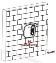
Step3. Use a  $\Phi$ 8 drill bit for the wall holes with 40mm deep, and insert 4  $\phi$  8\*60 expansion tubes, then put the top two expansion tubes into self-tapping screws (note: the top two self-tapping screws flange end distance is reserved about 6mm distance from the wall, can be used to open the key auxiliary calibration distance).
