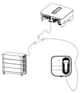
Connect inverter BMS port to "IN" port of waterproof connector via network cable labeled with "INV".
