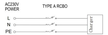
Diagram of electrical system of product (11kW/22kW):
