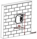
Step3. Use a marking pen to mark the 4 installation hole positions of the mounting accessory on the wall, and then drill 4 holes with a diameter of 8mm and a depth of 50mm on the wall using an impact drill, and finally use 4 M6 \* 50 expansion screws to fix the mounting accessory to the wall.
