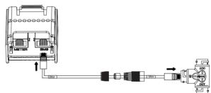
Connect communication port of battery to "OUT" port of waterproof connector via network cable labeled with "BMS".
