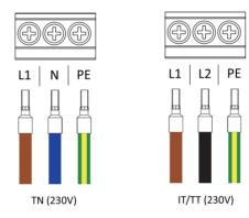
Different wiring modes of ECA-S11/22K-BS0 inlet lines are shown as below.
